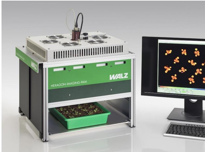
An aluminum bottom plate is used on the one hand to position a series of individual leaves in the focal plane or can also be used as a support for plant trays in a lower position. The focus of the 8 mm objective can thus remain at the same setting.
